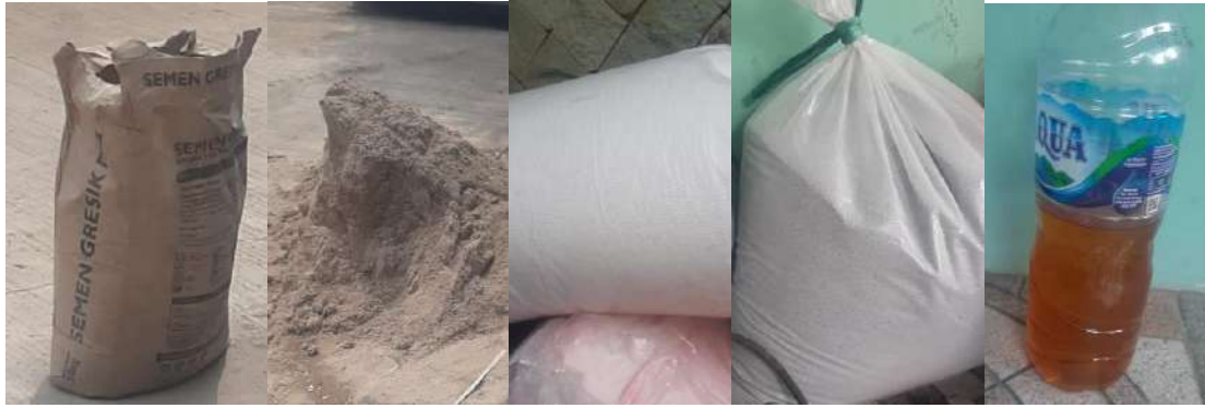
Gambar 4. Semen, pasir, steorfoam, silica fume dan superplasticizer
