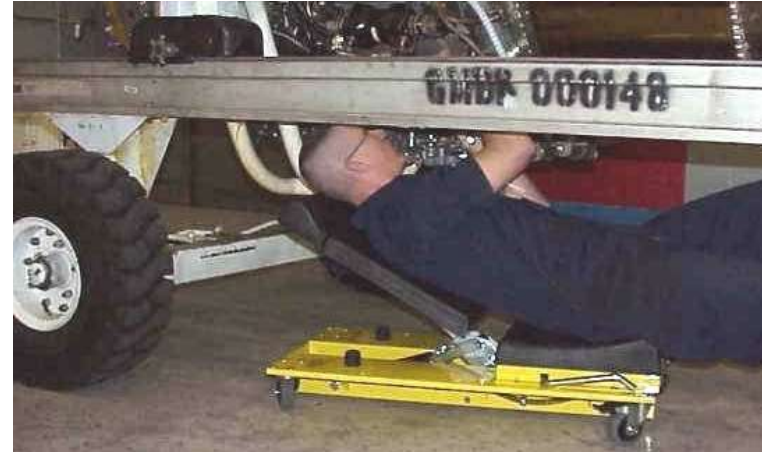
Ergonomic Improvement: Creeper supports mechanic and brings him closer to the task
