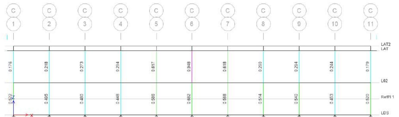
**Stress Ratio Kolom Beton Portal as C**
