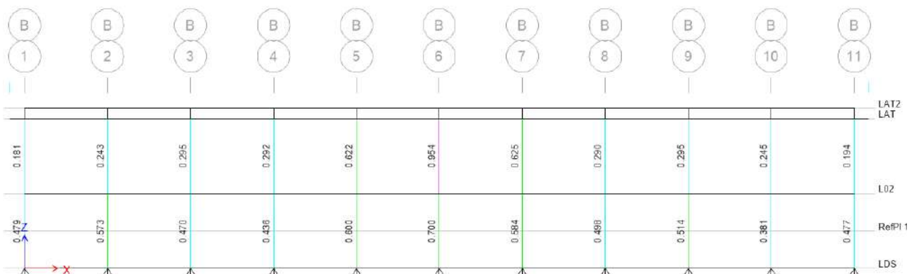
Stress Ratio Kolom Beton Portal as B
