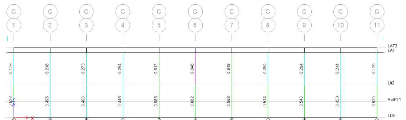
Stress Ratio Kolom Beton Portal as C
