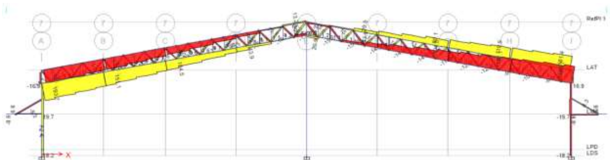
Gaya Dalam Aksial Tipikal Portal as 2 – as 15 akibat beban Gempa (kN)
