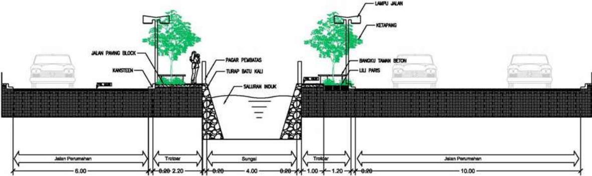
Gambar 15. Potongan D-D (Scale to Fit)
