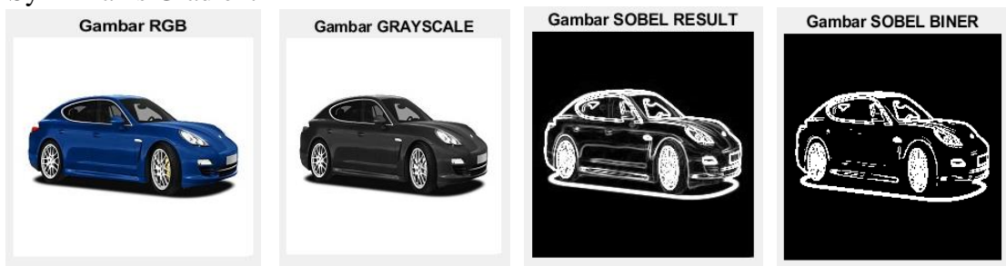
Figure 2. Transformation from RGB image into sobel image
