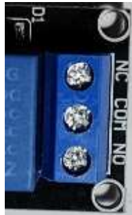
Gambar 4.5 Sisi Output Interface Modul Relay
