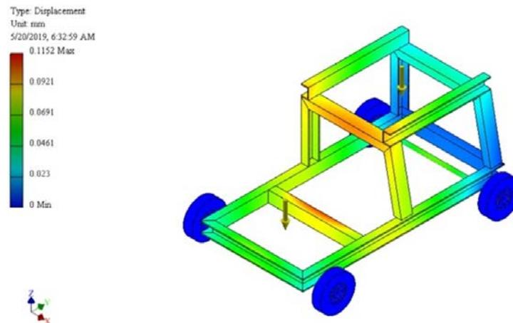
**Figure 4.** Deflection distribution of chopper machine construction [1], [2]
