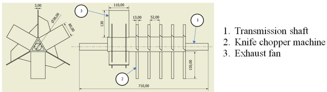
**Figure 2.** The knife of chopper machine design [1], [2]
