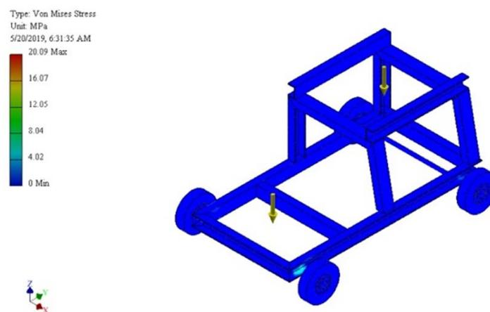
**Figure 3.** Stress distribution of chopper machine construction [1], [2]
