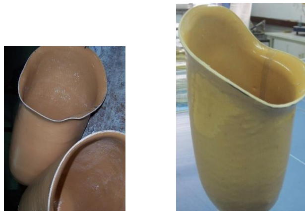
Figure 3. Socket product made from bamboo composites material
