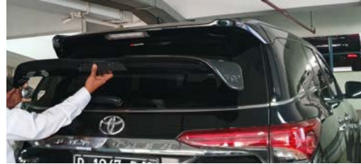
FIGURE 4. Spoiler Product Prototype with bamboo fiber composite material
