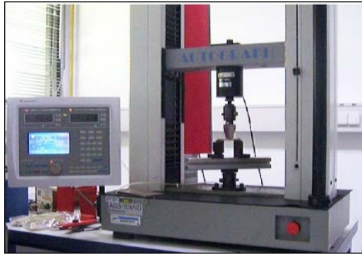
FIGURE 4. Bamboo Fiber Composite Flexural Test
