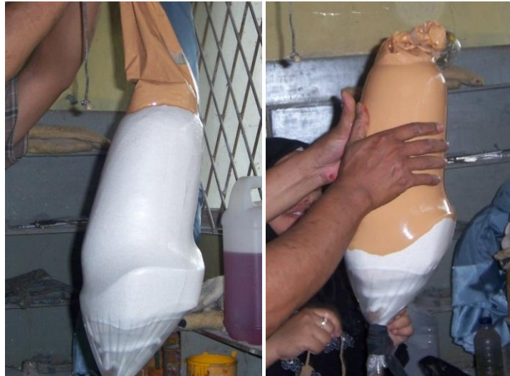
Figure 2. Manufacturing process of socket
