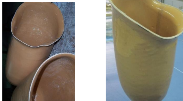
Figure 3. Socket product made from bamboo composites material
