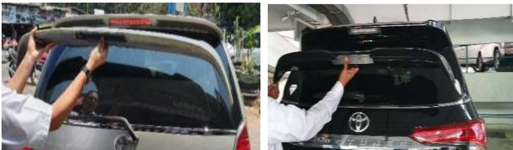
**Figure 4** Product prototyping of car spoiler using rattan fiber composite
