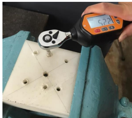
Fig. 6. Torque Testing on biodegradable bone screw
