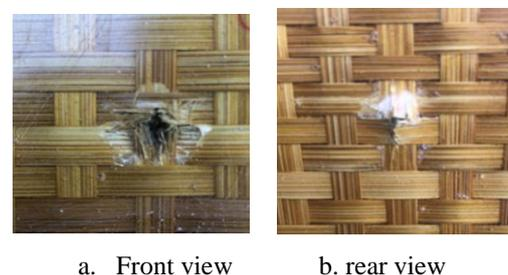
**Fig. 10.** Ballistic Test Results of the BSRECM  $0^0/90^0/0^0$  Laminate
