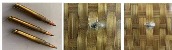
**Fig. 8.** Ballistic Test Results of the BSRECM  $0^0/0^0/0^0$  Laminate
