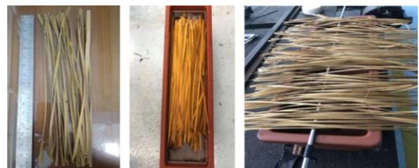
Fig. 1. Bamboo Strips Preparation
