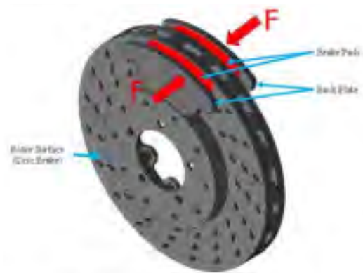
Figure 1. Force of friction between the brake pads and the rotor surface.
