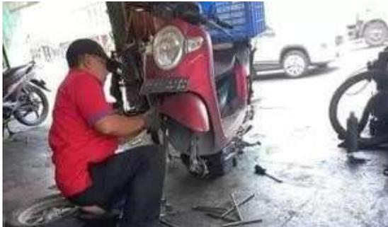
Gambar 1. Mekanis Mengecek Sokbreaker
