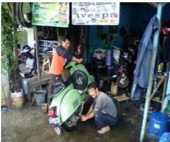
Gambar 8. Mekanik Mengecek Kic Starter
