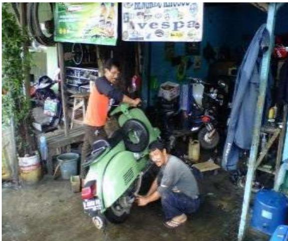
Gambar 3. Mekanik Mengecek Kic Starter
