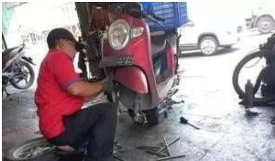
Gambar 6. Mekanis Mengecek Sokbreaker
