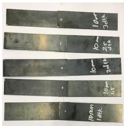
Figure.2 Steel Plate S45C
