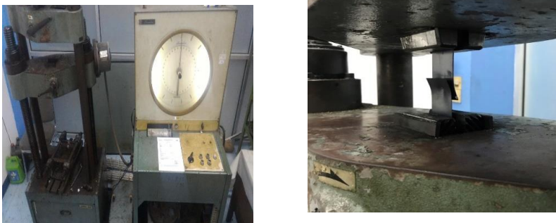
Figure .4 S45C Specimen Tensile Test
