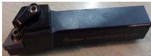
Figure 6. Tool Holder Cutting tool wear observations were made using a digital microscope.
