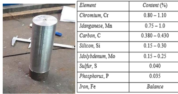
Figure 3. (a) AISI 4140 Steel Cutting force measurements using Force Dynamometer equipment
