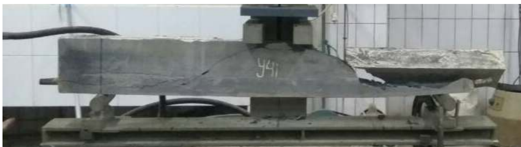
Figure 4. Shear failure pattern on beam
