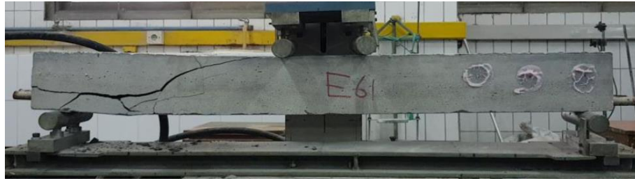
Figure 8 Beam E61 undergoes Shear Failure
