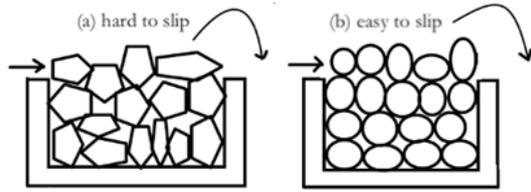
Fig.1 Comparison of the slip/crack strength of (a) angular coarse aggregate; (b) round coarse aggregate
