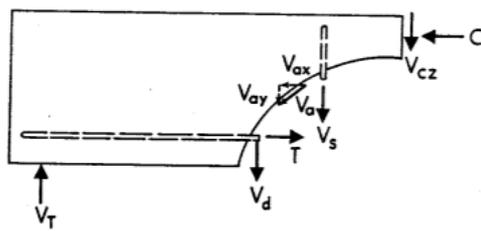
Fig.4 Forces acting at inclined crack [21]
