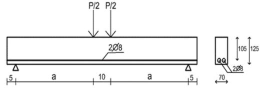
Fig.11 Beam details and experimental setup
