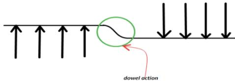
Fig.3 Dowel action on longitudinal reinforcement
