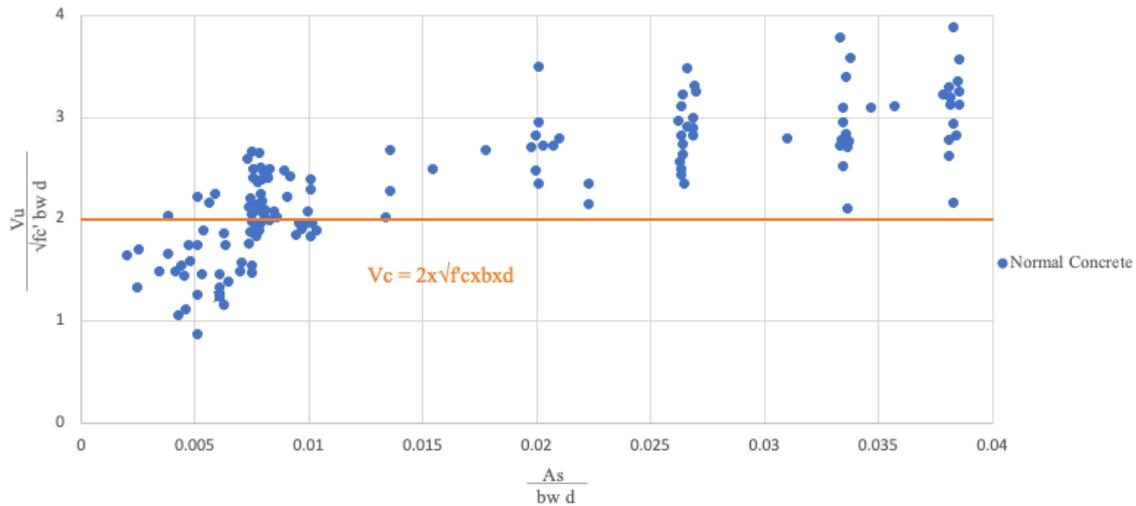
Fig.9 Influence of reinforcement ratio on the shear capacity of normal concrete [1].
