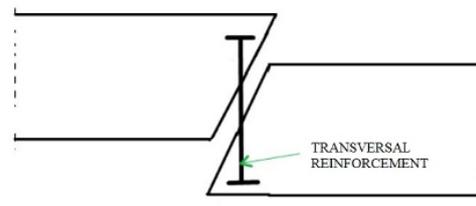
Fig.6 Shear cracks are held by transverse reinforcement (stirrup)
