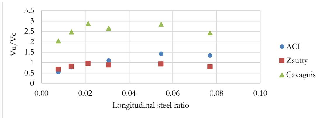
Fig.14 Relation between longitudinal steel ratio and  $V_u/V_c$
