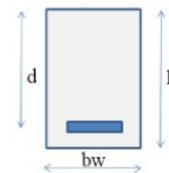
Fig.8 The beam's cross-section
