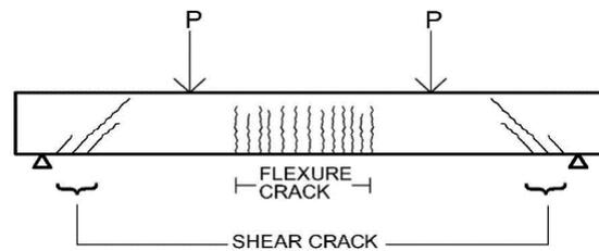
Fig.7 Cracks in concrete beam
