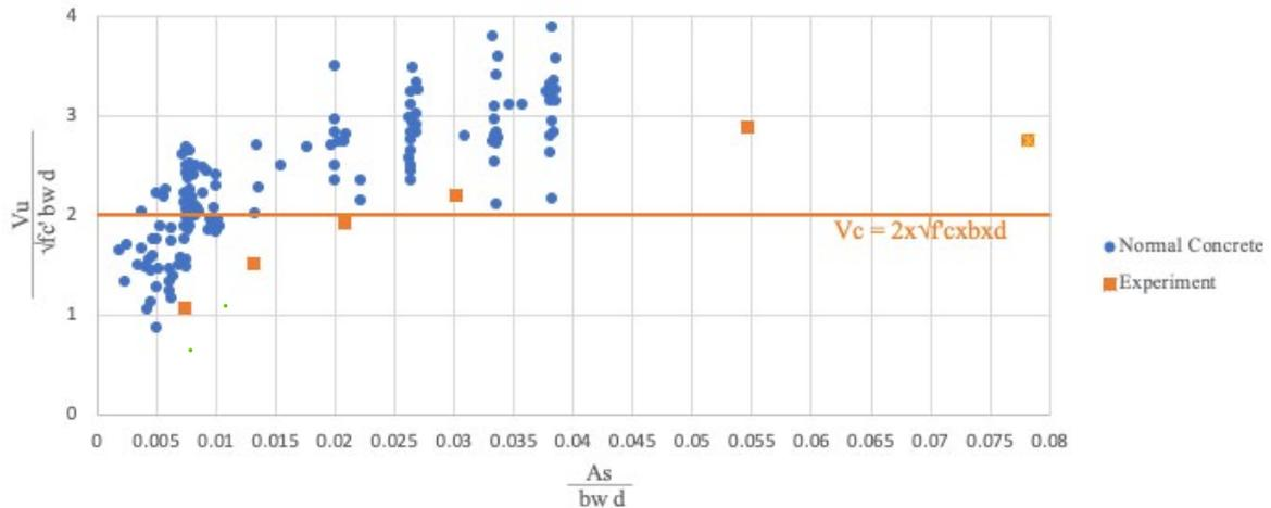
Fig.13 Effect of longitudinal reinforcement ratio, on shear capacity without stirrups
