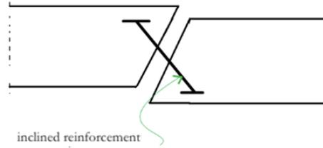
Fig.5 Shear cracks are held by an inclined reinforcement
