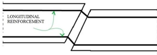
Fig.2 Shear cracks are held by longitudinal reinforcement
