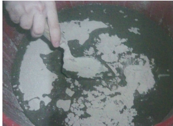
Figure 2. Mixing fly ash with activator solution
