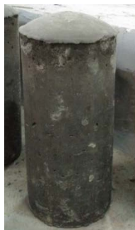
Figure 4. Volume alteration of geopolymer concrete
