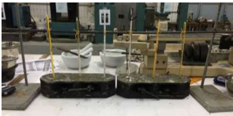
Figure 4. Temperature recording of cement pastes (from left to right: 0% – 5% of SA volumes)
