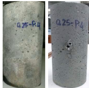
Figure 1. Specimen before (left) and after (right) immersion in sulfate.
