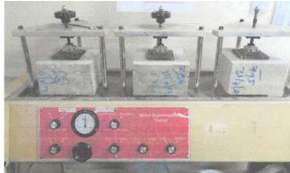
Figure 2. Specimens in the permeability test apparatus
