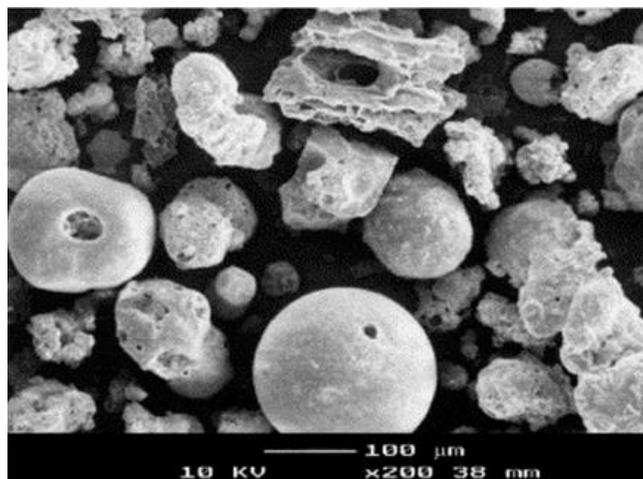
Gambar 7. POFA under microscope (Amran et al., 2021)
