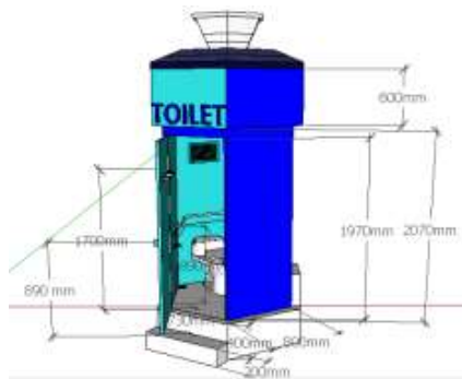
Figure 4. Dimension of 3D Design
