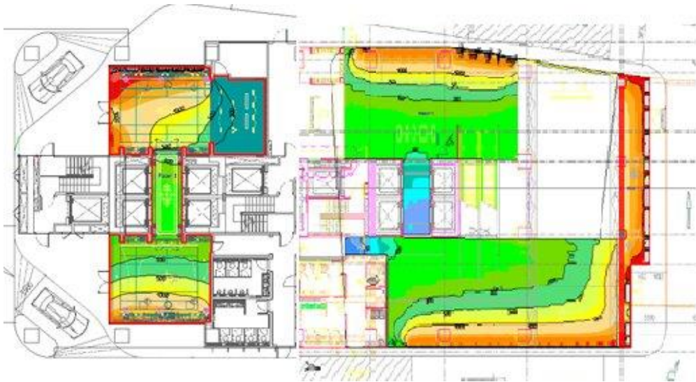
Figure 5. The sunlight in the afternoon that exceeds the recommended limits for a room causes a glare effect in the room.
