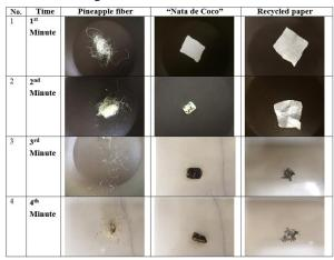
The findings on the heating process the material using Teflon on a stove with an internal temperature of 75-100 degrees Celsius for 1-5 minutes until saturated exposure refers to the following:
