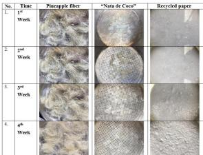
The findings in the form of the drying process in the form of direct exposure to sunlight for 30 days in tropical Jakarta temperatures vary from 22 degrees Celsius to 38 degrees referring to:
