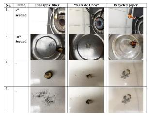
The findings on the roasting process using blue-orange fire with a temperature of 1000-1500 degrees Celsius to produce the following references:
