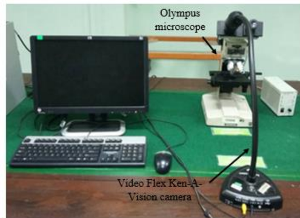
FIGURE 6. Olympus microscope equipment used to analyse solder joint
