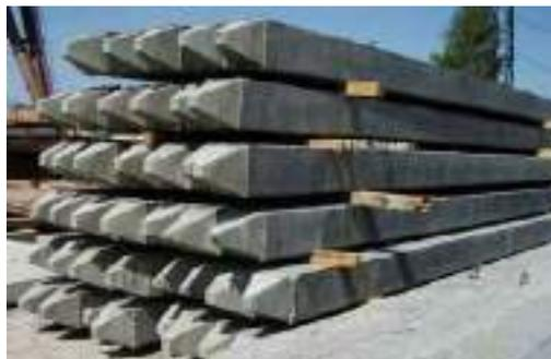
Gambar 12.16 Tiang Beton Pracetak [7]
