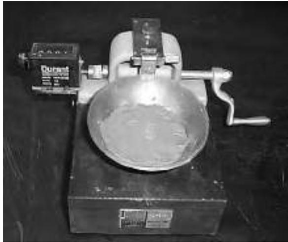
Gambar 11.9. Alat pengujian *Atterberg Limit Test* [6]
