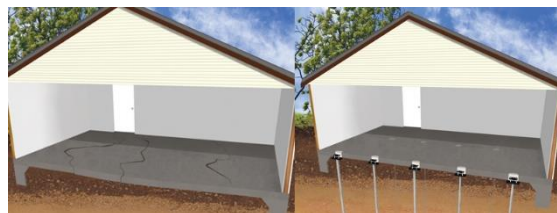
Figure 1. Settlement that occurs in slab-on-ground. ( https://www.alsplumbing.com/low-priced-slab-leak-repair-no-bargain/foundationrepairhousediabramwithwihoutpiers/ )
