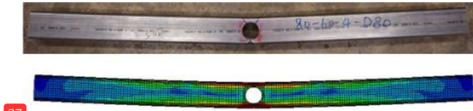
37 Fig. 5. Comparison of failure mode obtained from the test and FEA for specimen 80×60×4D80.
