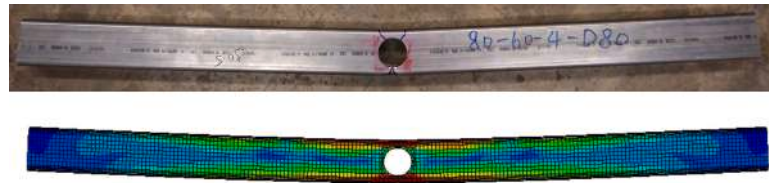
Fig. 5. Comparison of failure mode obtained from the test and FEA for specimen 80×60×4D80.
