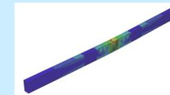
Gambar 10. Model Keruntuhan L300x120x2D20T24
