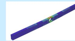
Gambar 13. Model Keruntuhan L300x120x2D90T24
