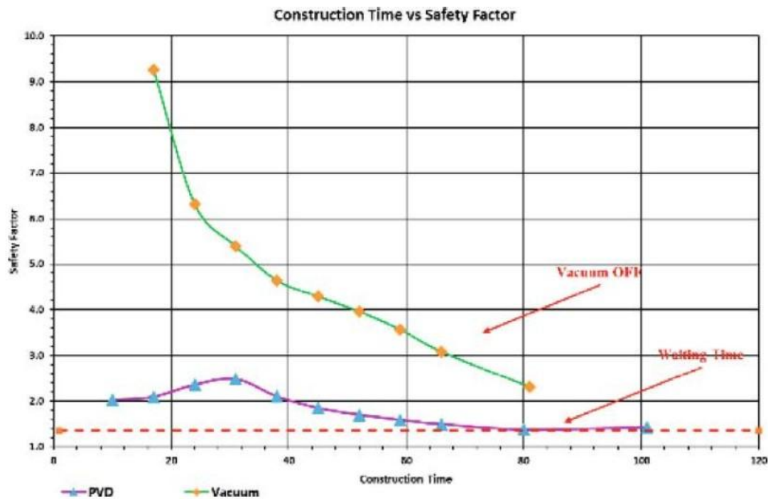
Fig. 6 Comparison of construction time against factor of safety values
