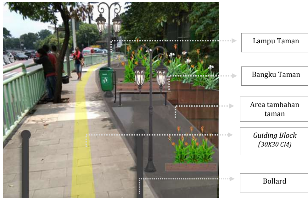
Gambar 4.28. Penataan Segmen 1 (Area 2) (Sumber : Peneliti,2020)
