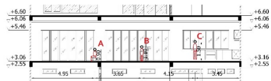
Figure 6 Light Intensity Measuring Point Height (Source: Personal Documentation, 2021)
