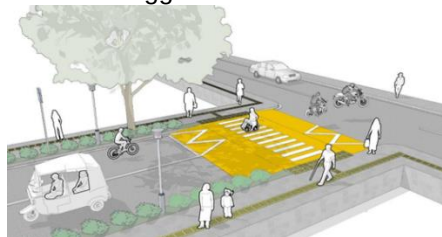
Gambar 1. Contoh pedestrian platform di persimpangan (Sumber : Kementerian PUPR, 2023)
