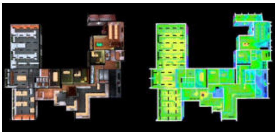
Figure 2. Example of calculation of DIALux Source: https://www.dial.de/en/blog/article/lighting-designer-tom-van-roey-on-DIALux/ , 2020
