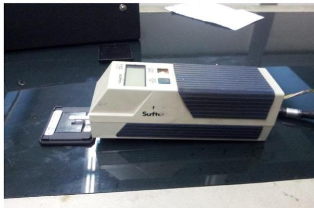
Gambar 7. Surface Tester Mitutoyo 211
