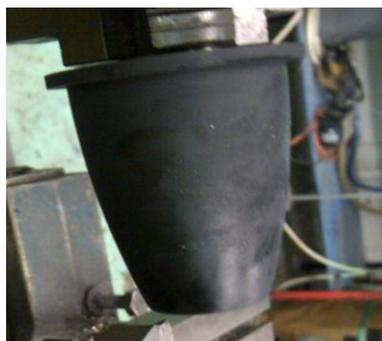
Gambar 5. Elektroda Graphite
