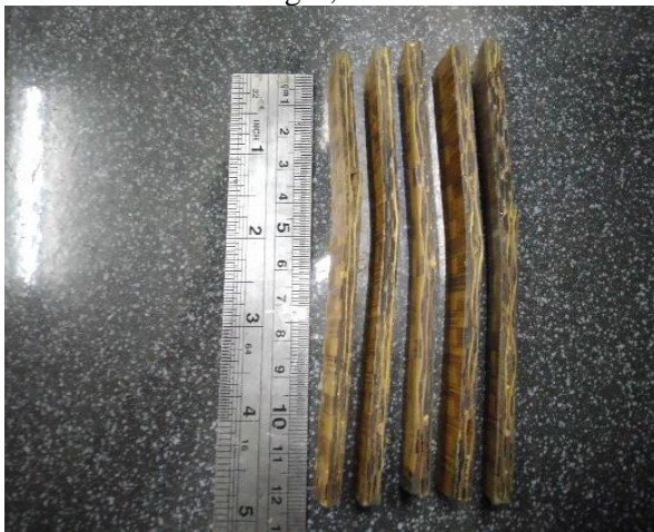
Figure 1. Compressive Test Results on Specimen A
