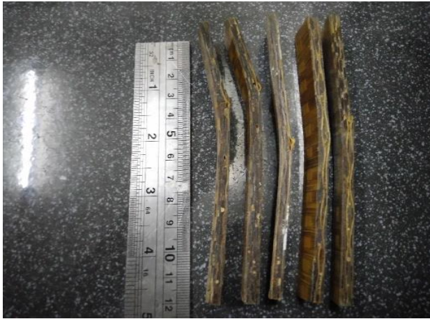
Figure 3. Compressive Test Results on Specimen C
