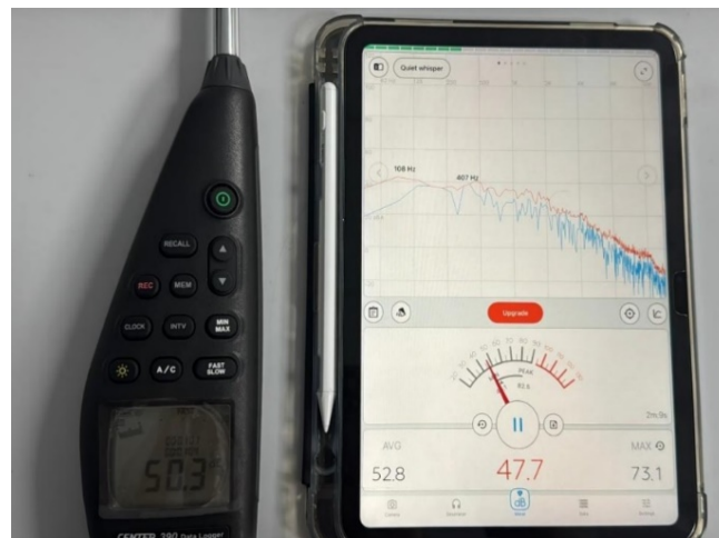
Fig. 3. Calibration Setup Using iPad and Sound Level Meter
