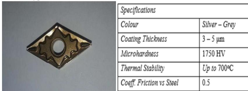
**Figure 5.** Coated Carbide cutting tool type DNMG 150404 The cutting tool insert is attached to the tool holder
