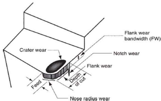
**Figure 1.** Flank and Crater Wear of Cutting Tools [7]
