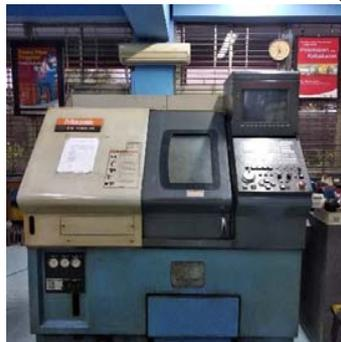
**Figure 2.** CNC Lathe "Mazak Mazatech *Quick Turn 8N*" The workpiece materials are AISI 4140 Steel
