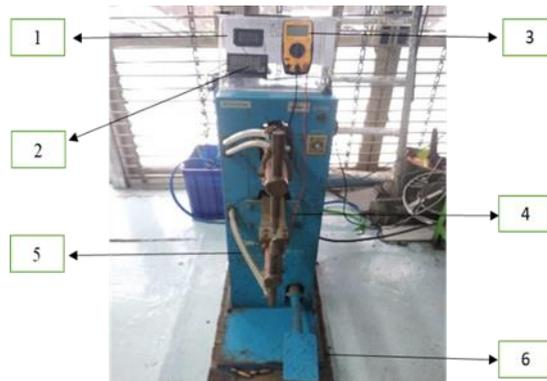
Gambar 3.1 Mesin *Spot Welding*
