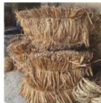
Fig. 1. Dried WH Stem used as the Main Material of the "Adjustable Chair".
