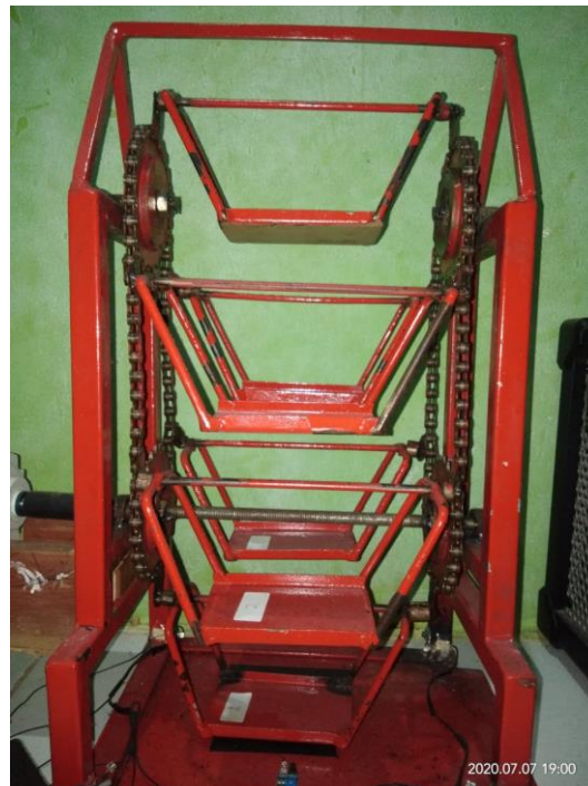
Figure 4. Realization of the designed rotary parking system model
