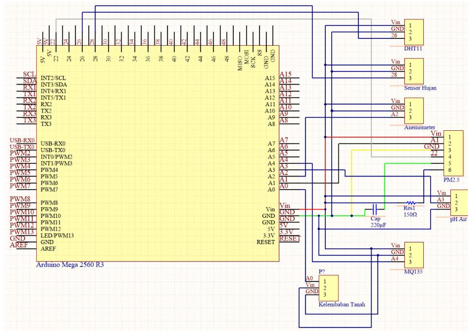
FIGURE 2. Schematic diagram of a whole system circuit.
